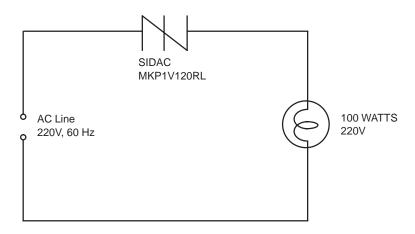
This is done in order to lower the RMS voltage to the filament, and prolong the life of the bulb. This is particularly useful when lamps are used in hard to reach locations such as outdoor lighting in signs where replacement costs are high. Bulb life span can be extended by 1.5 to 5 times depending on the type of lamp, the amount of power reduction to the filament, and the number of times the lamp is switched on from a cold filament condition.
