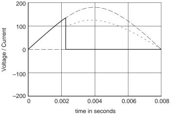
In this case, the conduction angle is around  $130^{\circ}$  (6 msecs) in each half cycle of the sinusoidal current waveform, therefore, the average power of the lamp can be obtained by calculating the following operations:
