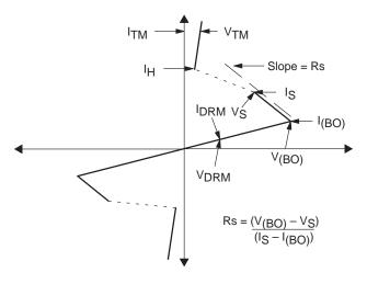
Once the input voltage exceeds V(BO), the device will switch on to the forward on–voltage VTM of typically 1.1 V and can conduct as much as the specified repetitive peak on state current ITSM of 20A ( $10\mu$ s pulse, 1KHz repetition frequency).
