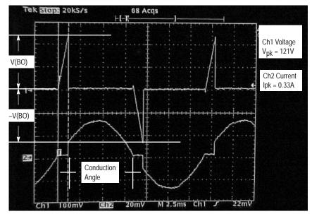
In both previous cases, once the ac line voltage reaches the V(BO) of the SIDAC (MKP1V120RL), it allows current flow to the incandescent lamp causing the turn–on of this at some specific phase–angle which is determined by the SIDAC because of its V(BO).
